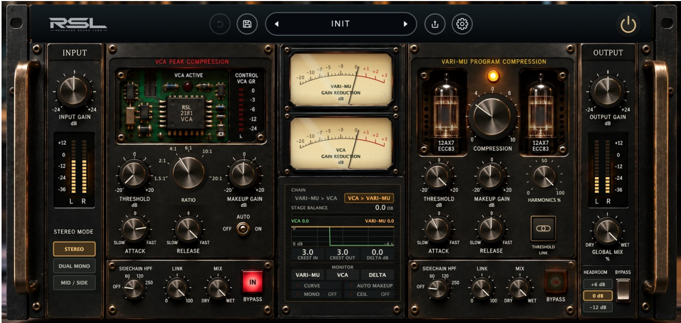
RSL Bastion at rest, in its default order: the VCA stage on the left, the Vari-Mu stage on the right. Swap the order under CHAIN and the two panels trade places.
