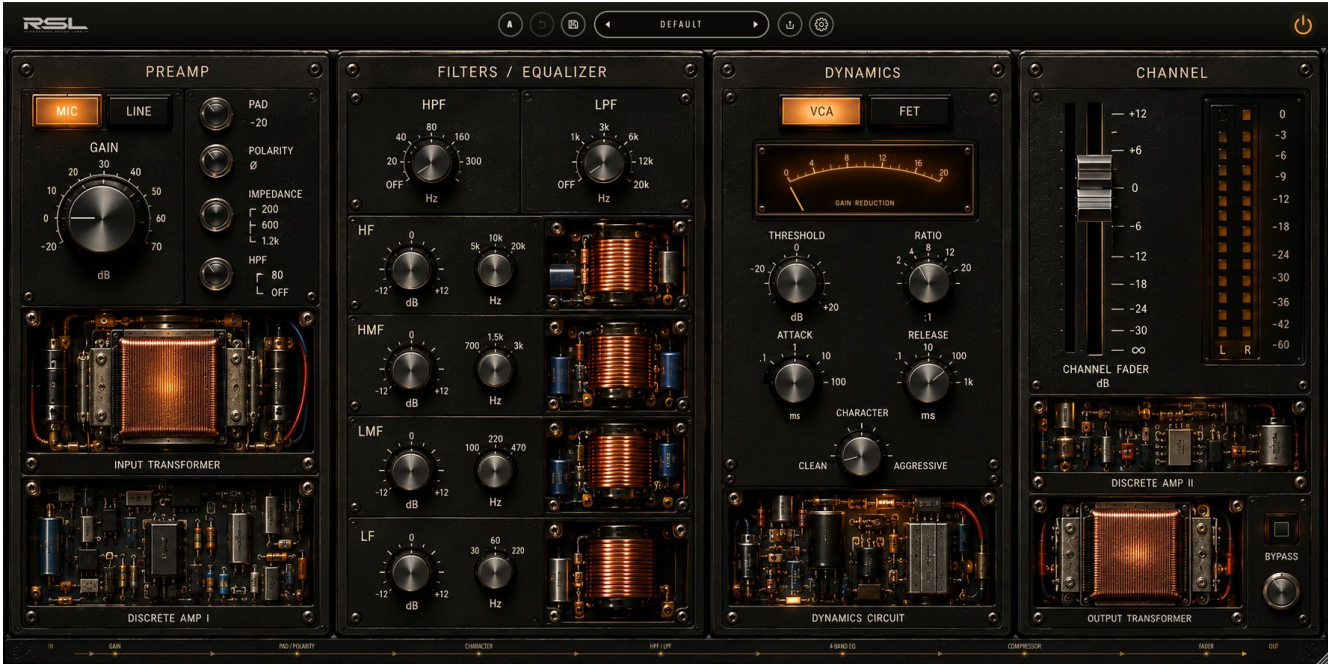
RSL Channel at its defaults. The signal runs left to right through four panels: PREAMP, FILTERS / EQUALIZER, DYNAMICS and CHANNEL.
