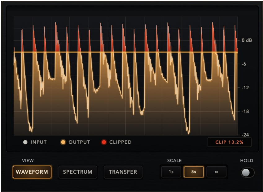
WAVEFORM at 5s, with the threshold line at -3 dB and the CLIP readout bottom right.
