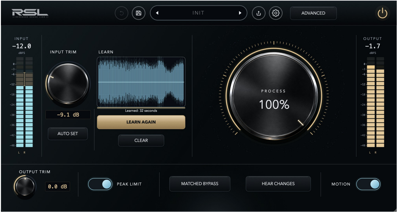
The faceplate reads left to right as the three steps: Input, Learn, Process. The utility strip along the bottom holds output and monitoring.
